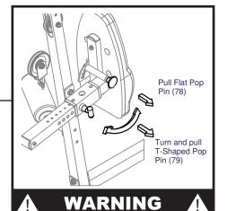
Pay special attention to the plunger on Pop Pins (78) and (79). Always be sure that the plunger is **fully engaged** into the hole you select. Also, be sure that the spring in Pop Pins (78) and (79) operates freely. Failure to do so may result in death or serious injury.
