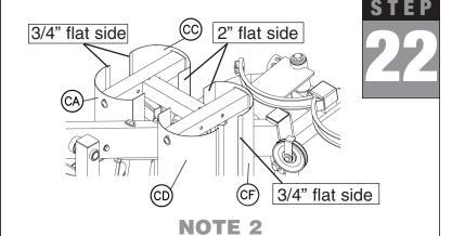
This is the top view of the four Weight Stack Shrouds. Note the shape of each shroud for proper placement.
