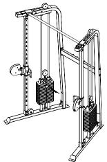
Above shows step 4 assembled and completed
